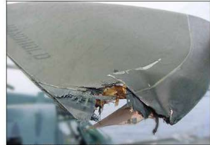
Tip Strike on AW101 Blade (Crown Copyright)
